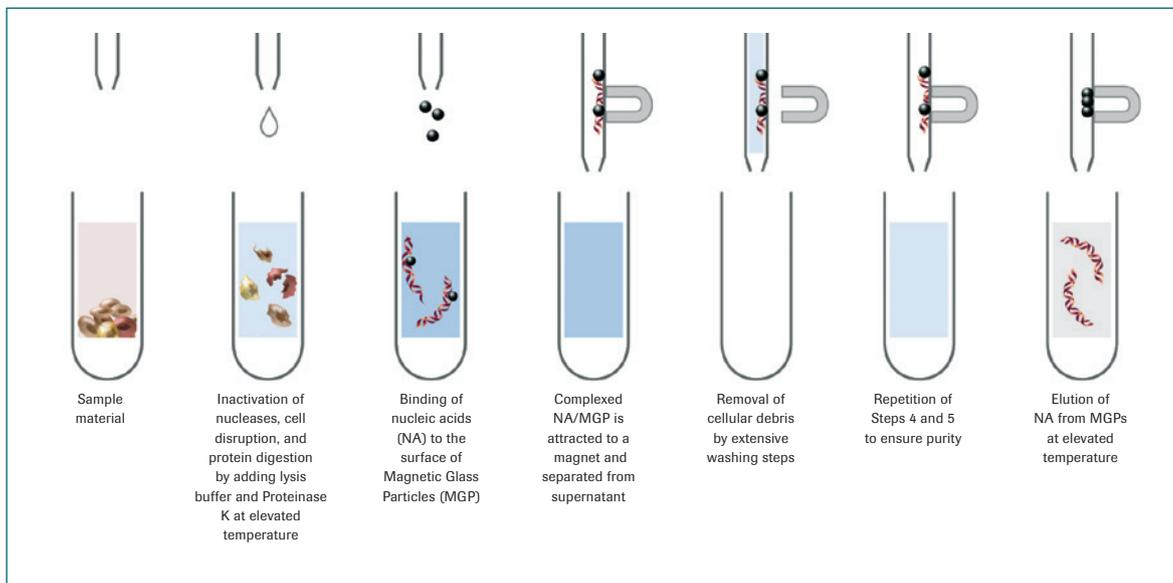
▲ **Figure 1: Overview of nucleic acid isolation and purification with the MagNA Pure LC System.**
