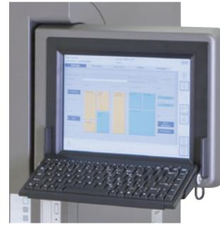
The MagNA Pure LC 2.0 System is operated by a convenient touch-screen user interface and an integrated PC. It combines on the same platform the purification of nucleic acids from biological samples, as well as the set-up of PCR reactions. This makes the MagNA Pure LC 2.0 System a true “walk-away” system.
